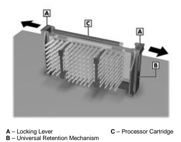
**10.** Install the replacement processor cartridge (see "Installing the Celeron or Pentium III Processor Cartridge" in the following subsection).
